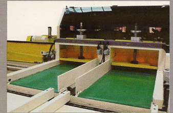
Twin table designed doubles the output capacity of the line
