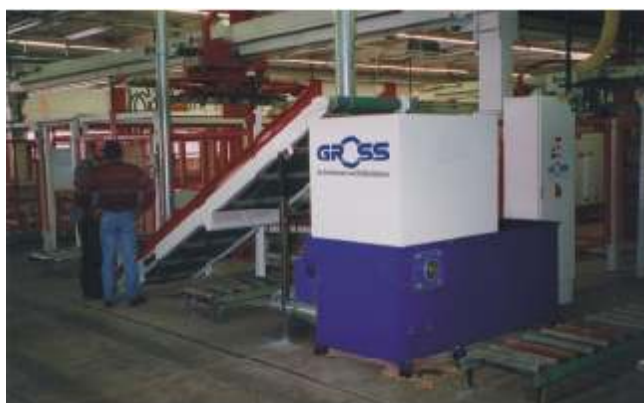
GAZ 82 with customer specific hopper (sound proofed, double skinned)
