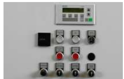
The PLC controls ensure user friendly, fully automatic operation Option: with info display
