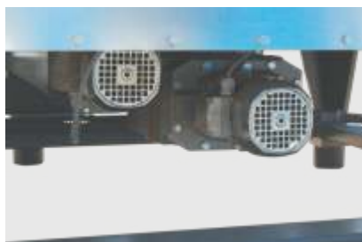
Two high-powered motors drive the screw compressor and the supercharges unit
