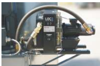
Option: Oil cooling system for the hydraulic unit
