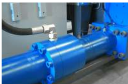
Strong pressing operation by amply dimensioned cylinder
