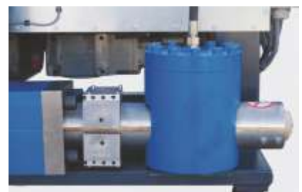
Option: cooling system for the presstong
